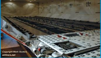
**Gillfloor® 4518**, qualified to BMS 4-17 Types X and XI, is a lightweight, high-strength floor panel made of unidirectional and woven glass reinforced epoxy facings, bonded to para-aramid honeycomb core. Gillfloor®4518 is installed in the main deck floor locations of the B777 freighter aircraft.
