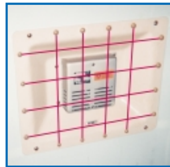
Fiberglass reinforced phenolic resin housing for smoke detection equipment in baggage compartment
