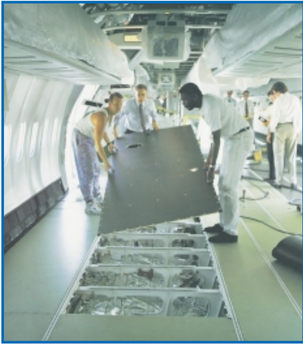
Installing an M.C. Gill fabricated flooring panel in an MD-11
