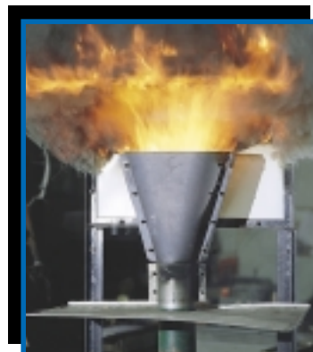
Oil Burner-Burn Through Cargo Liner Test
