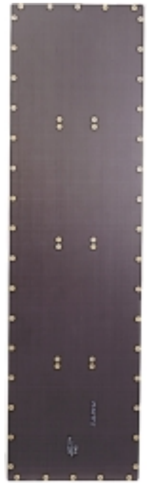
Carbon/Nomex fabricated floor panel
