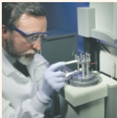
The dynamic mechanical analyzer determines the mechanical properties of a material as a function of temperature. Dr. Terry Creasy, Assistant Director of the Composite Center, demonstrates the loading of the sample.
