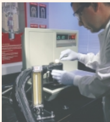
The primary purpose of this thermogravimetric analyzer is to determine the onset of degradation. The operator is Hongbin Shen.
