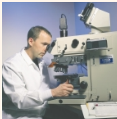
The high-power light microscope allows maximum magnification of polished polymer and composite samples through one of the five turrets. A real-time digital camera captures images for analysis of parameters such as fiber volume fraction.
