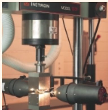
Quartz lamps enable this Instron machine to test in tension or compression (shown) at temperatures as high as 2500°F while heating the samples within seconds.
