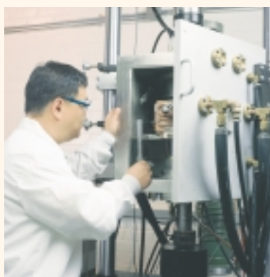
Graduate student Chanman Park inserts a coupon to test for tension fatigue and stress rupture of ceramic matrix composites.
