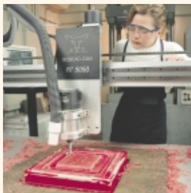
The CNC profiler is used to make tooling and patterns for contoured parts. The operator, Ms. Siari Sosa, is a Ph.D. candidate.
