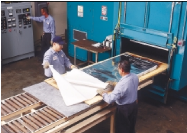
The Dielectric Press greatly shortens curing time.
