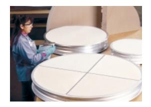
A Desiccant Air Conditioning System removes moisture from ventilation system air, making it easier to cool. The term "desiccant" means "drying agent." This system can translate into significant energy savings because it takes less energy to cool *dry* air than to cool *humid* air.
