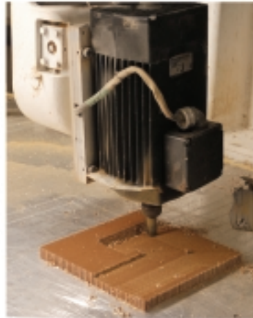
A CNC machine profiling a piece of honeycomb
