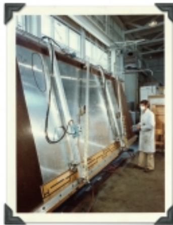
The Walking Man testing machine puts flooring through its paces
