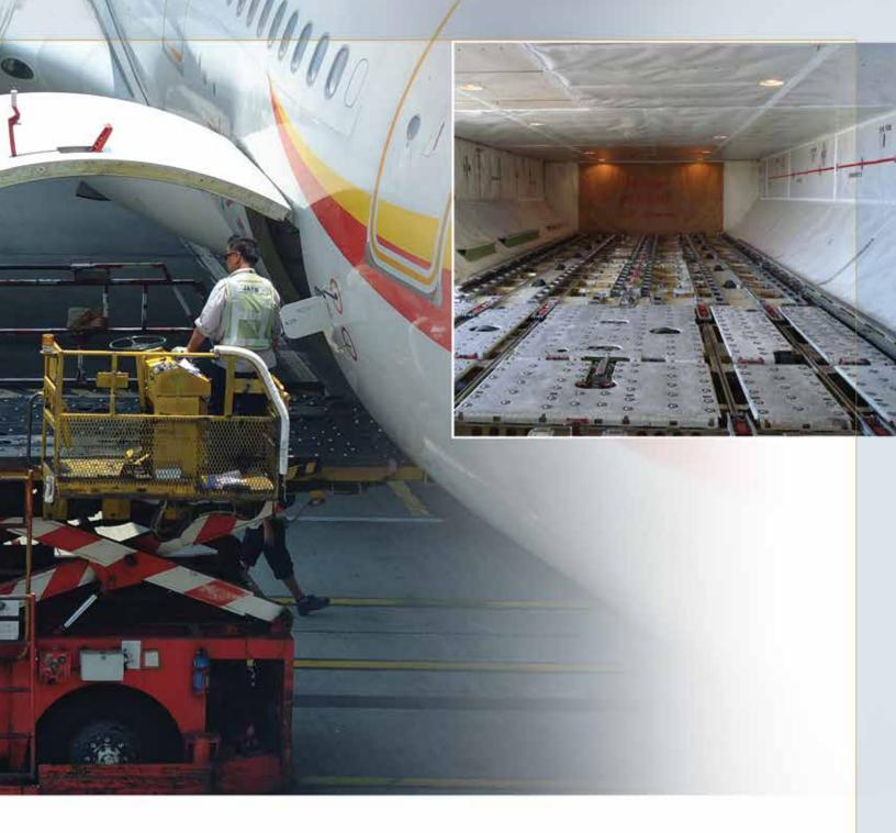
**Gillfab 1367/A** is qualified to BMS 8-223 Class 2 Grade B. It is a high-impact-resistant phenolic cargo liner that also offers low fire, smoke, and toxicity characteristics.
