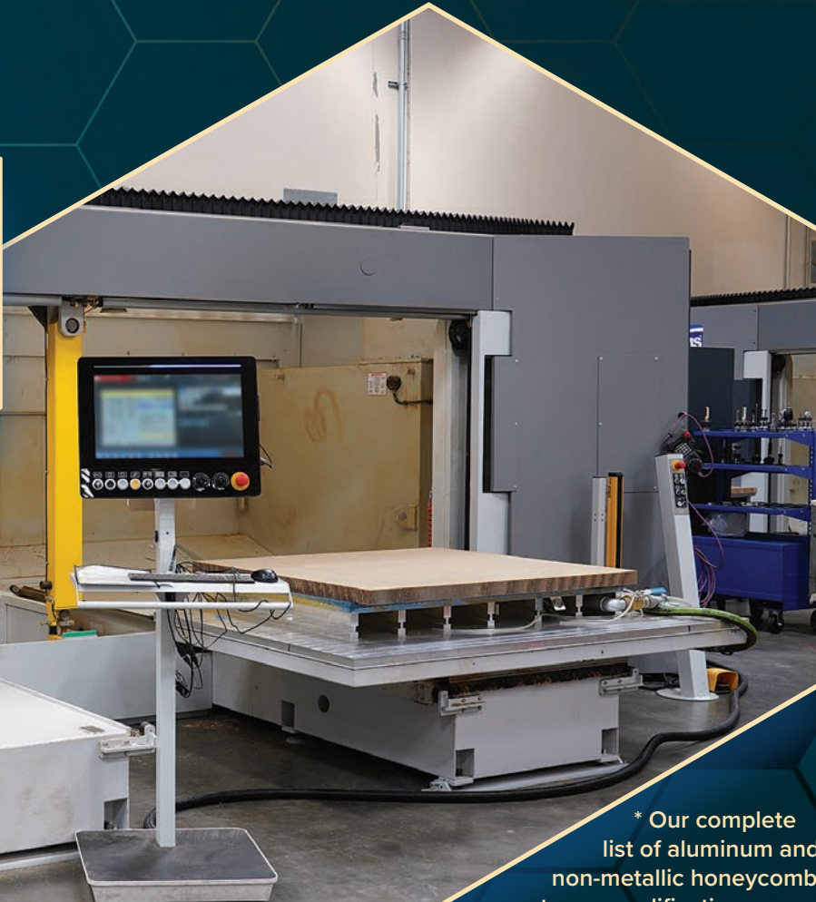
Non-metallic core is heat-formed, potted and 5-axis machined for flap track fairings.
