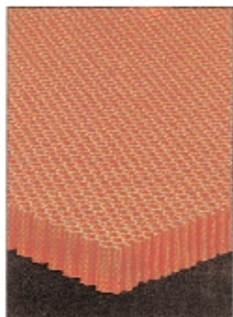
Specially formulated phenolic resin impregnated in aramid paper boneycomb core — used as the core material in a variety of aircraft flooring and other sandwich panels.
