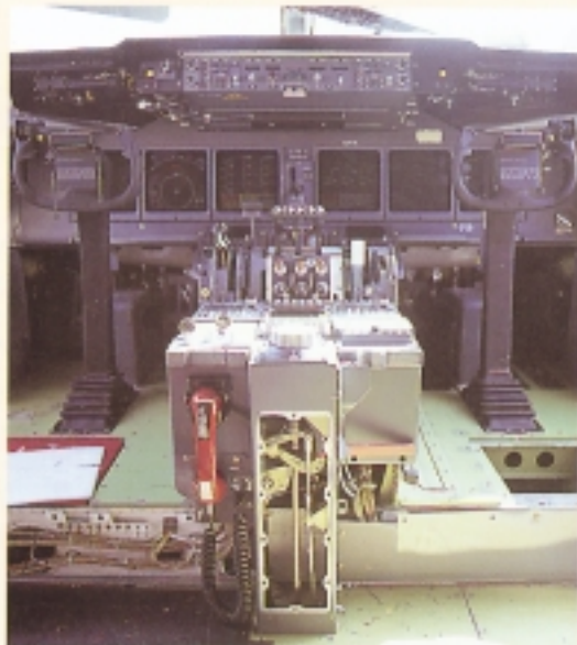
A view of the cockpit interior showing the avionics and 4109 flooring. (The green primer on some of the panels was applied by McDonnell Douglas, but is not required.)
