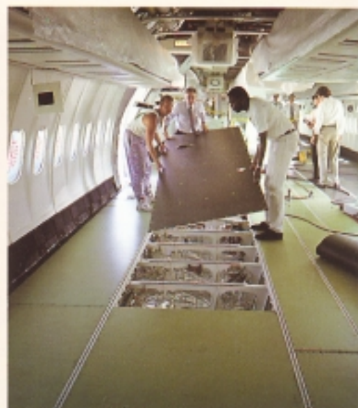
McDonnell Douglas employees Jeff Bartlett (left) and Reggie Hill installing one of the very first 4109 flooring panels in an aisle.
