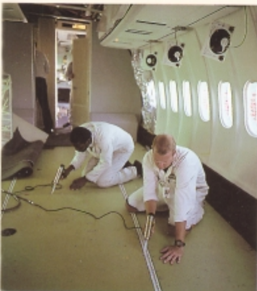
Sealing a forward flooring panel using polysulfone applied with an air powered caulking gun.
