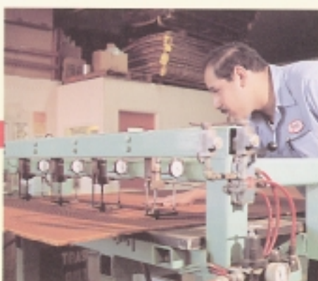
The entire slice goes to a dial indicator table and thickness is measured along the entire length. Slices of the same thickness, density and cell size then await sandwich panel production. Each slice is tagged for traceability.
