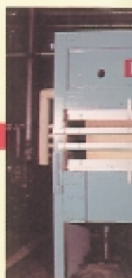
Stacks of printed Nomex paper under pressure to be pressed. A separate step, pin pressing, is required prior to the final pressing process.
