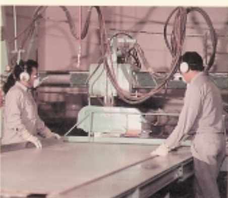
This panel is being cut and trimmed. From here it goes into finished goods inventory or to shipping.
