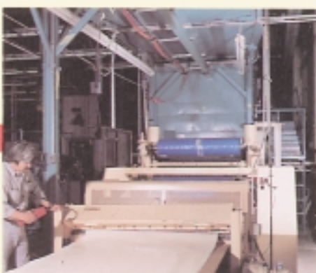
The resin impregnated facing comes out of the B stage curing oven and is sliced to pre-determined length. It then goes into refrigerated storage to await sandwich panel construction.
