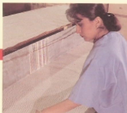
Stacking the individual sheets of printed Nomex paper, a critical step. Glue lines of one sheet cannot be placed directly over glue lines on the sheet below.
