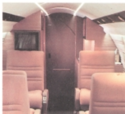
The versatility of sandwich panels used for aircraft cabinetry is illustrated by the pictures above. From left to right, the sides, top and bottom of a food
