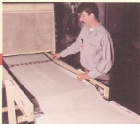
Printed Nomex paper comes out of the printer where it is sliced and stacked in piles of 100 sheets, preparatory for loading the press.
