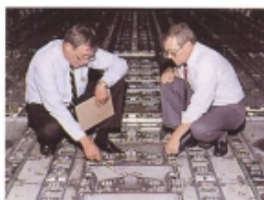
Fiberglass faced/balsa core sandwich panels for flooring resist high abuse in Federal Express 747 cargo compartments.
