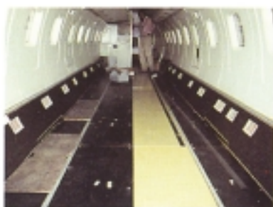
In the Embraer EMB-120 highly rigid (black) sandwich flooring is installed in the aisle; less rigid (yellow) panels under the seats.
