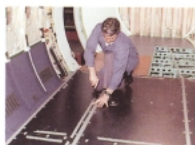
British Aerospace employee installing graphite faced/Nomex honeycomb flooring in the BAe 146 passenger area.
