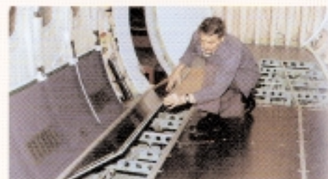
A section of 4109 flooring being installed in the BAe 146-200.
