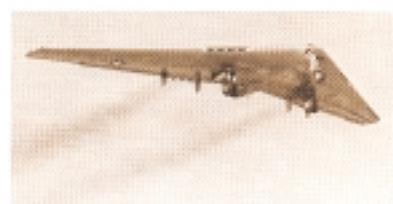
Jet powered YB-49 on a test flight take-off October 1947. Four inlets on each side of the wing admitted air to the submerged engines.
