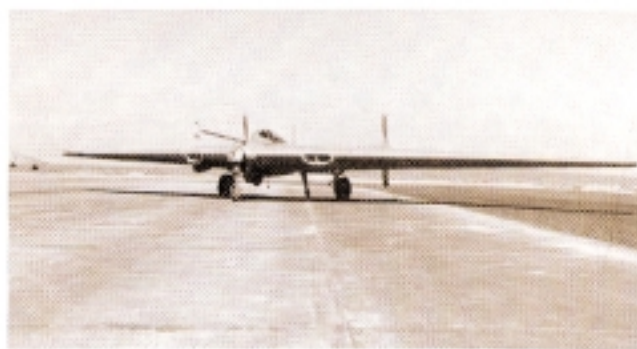
The primary mission of these scale models was to provide flight test information from which performance data for the XB-35 could be predicted.
