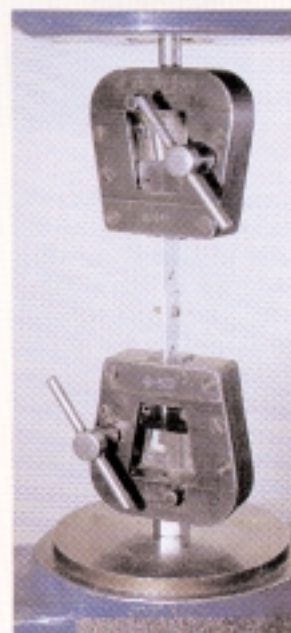
BOLTED JOINT PULL-OUT TEST measures the cargo liners edge bearing resistance to force.
