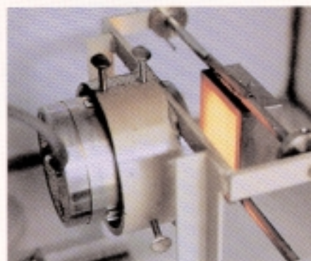
NIST (NBS) SMOKE CHAMBER TEST measures smoke density of cargo liner when exposed to heat and flame.
