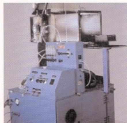
OSU HEAT RELEASE TEST measures the amount of heat dispersed over a given dimension in fire conditions.
