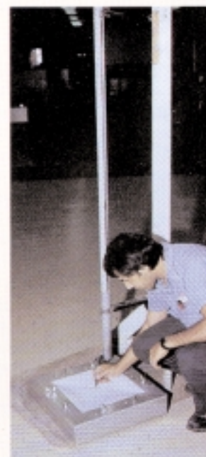
IMPACT OR PUNCTURE RESISTANCE TEST indicates the cargo liner's ability to withstand penetration.
