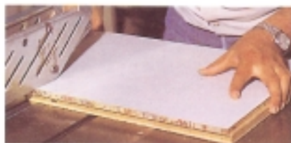
This panel is being cut on a table saw using a diamond grit blade with a backing piece (in this case, plywood) under the panel.
