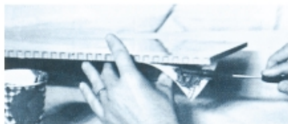
Edge delamination — coat both skin and core with carefully mixed epoxy adhesive. Always apply pressure while adhesive cures.
