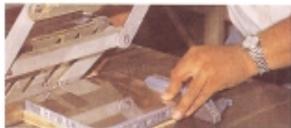
This panel is being cut on a table saw using a carbide tip blade with a backing piece (plywood) under the panel. (Note: the blade guard on the saw has been raised for purposes of photographic clarity only. O.S.H.A. and standard safety procedures dictate this blade guard remain in a down position at all times when the saw is in use.)
