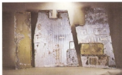
These corroded aluminum flooring panels were removed from the galley of a DC9. This amount of corrosion is typical for aluminum in "wet" areas. Gillfloor 5166 eliminates this type of failure.
