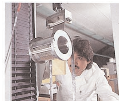
The climbing drum peel test measures force required to separate facing from core; also strength of the adhesive.
