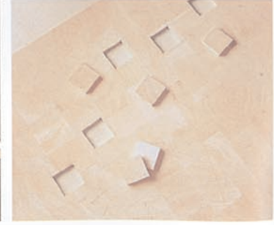
This sample sheet of end grain balsa shows the number of samples that have been cut out for routine Q.C. density checks.
