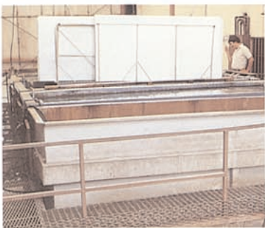
Aluminum sheets for sandwich panel facings are cleaned in these 54" x 174" tanks into two different solutions.
