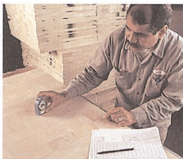
Balsa saw operator tests slice for proper hardness. This screening test will indicate if further testing is necessary.
