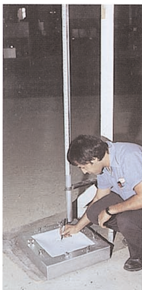
Impact or Puncture Resistance Test indicates the cargo liner's ability to withstand penetration.
