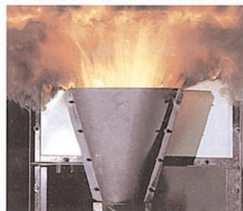
Burn-Through Test. If flame burns a hole through the test specimen, the test is considered a failure.
