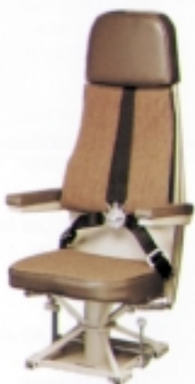
This observer's seat is designed to withstand 16 G's in each of five directions.
