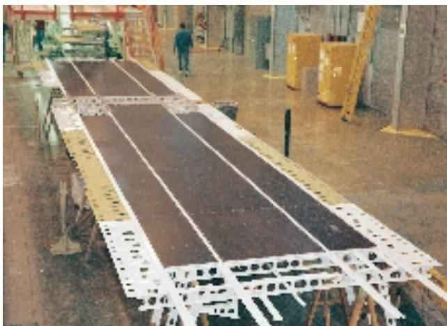
Gillfab 4109 panels installed in the flooring assembly at Douglas' Salt Lake City plant.
