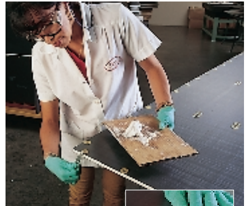
Technician smoothens the edge fill compound and ensures there are no air bubbles along the panel's edges.
