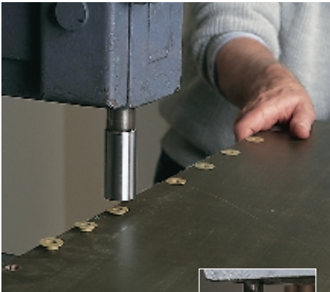
Technician adjusts panel on the roller table to ensure proper alignment of inserts. Then inserts are firmly set into the panel.
