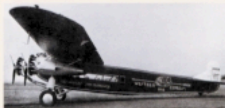
The Fokker F-10 Twelve-passenger Monoplane.
