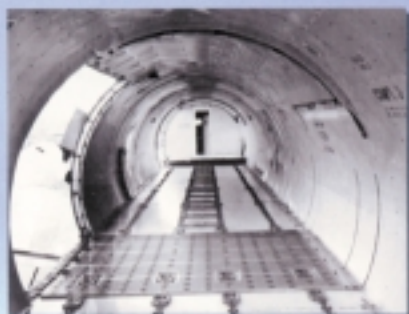
Interior of Lockheed Electra freighter conversion using M.C. Gill cargo liner.
