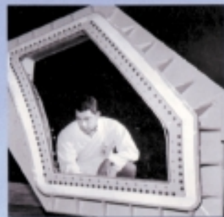
Giffab 1009, a nylon cloth/acrylic resin laminate used as edging to provide strength for attachment to aircraft.
