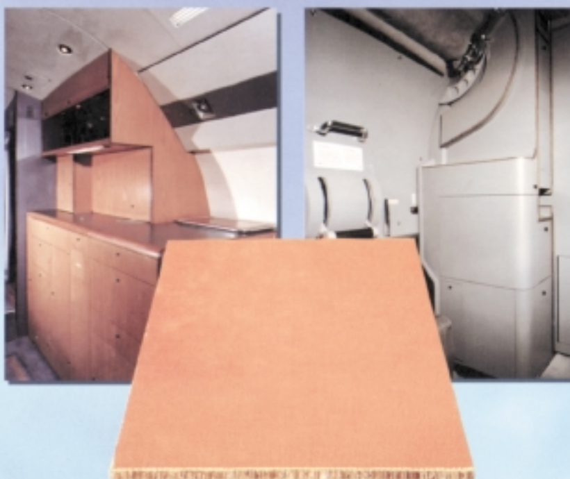
The Falcon 90 uses Giffab 5055 for the interior cabinetry shown below.
