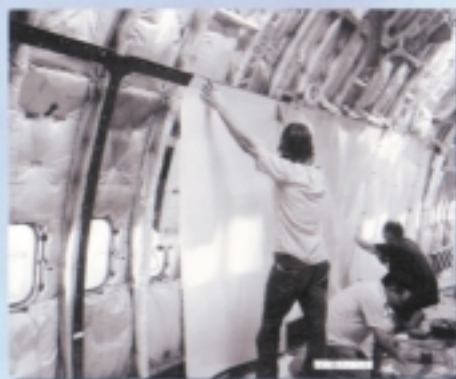
Gylliner 1438 being installed in 747 freighter conversion.
