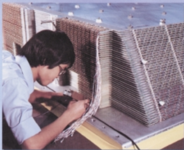
As part of a research study of sub atomic particles, including the Quark, Lawrence Livermore Laboratory sought M. C. Gill's assistance in designing and manufacturing 72"x 149" flat panels with pure lead cores, fiberglass interlay and aluminum foil facings. Here a technician wires electrical connections to the panels.
