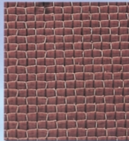
In response to customer requests, overexpanded Gillcore is now available. It facilitates curving or forming the honeycomb into simple contours in the "W" (warp or width) direction.
