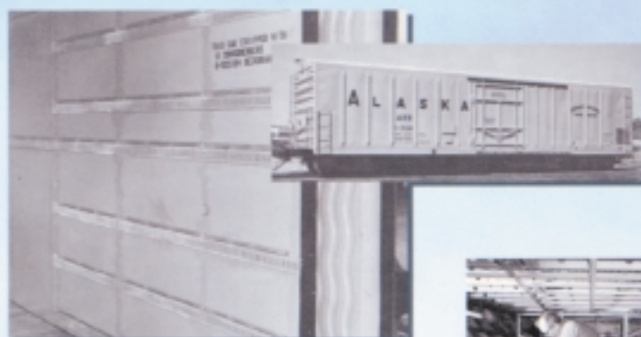
Gylliner 965, a 1/32" glass mat bonded to exterior grade plywood, was made especially for Alaska Railroad to line the interiors of their refrigerated boxcars. The cars carried fresh and smoked meats, vegetables, and other produce.
