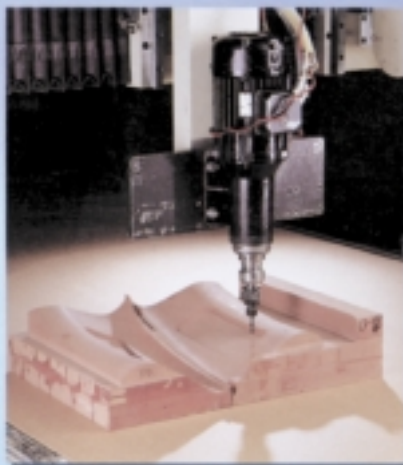
The CNC machine profiling a pattern used to make molds for contoured parts.
