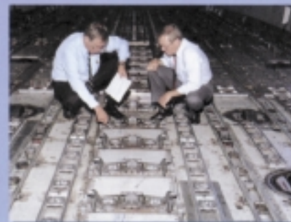
One of the periodic checks on in-service wear—in this case, Giffloor 5007C in a FedEx 747 freighter.
