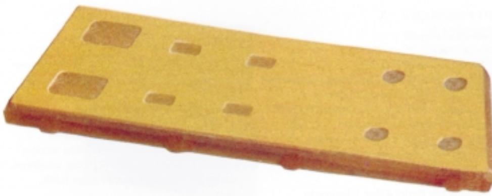
Gillfoam molded as a core material for an automotive flooring panel. Its light weight, beat resistant characteristics, and the ability to mold it in almost any configuration make it the material of choice for many components of today's modern transportation needs, be they for automobiles, aircraft, light or heavy rail, or marine.
