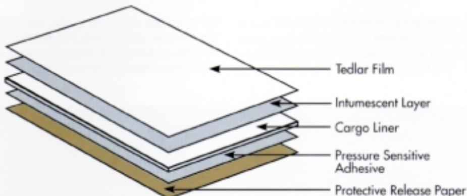
The Tedlar overlay can be cleaned, increases resistance to moisture damage, provides continuity of surface finish, uniformity of color, and after installation makes any subsequent damage to the patch easier to see. The intumescent coating completely covers the patch material and provides an excellent thermal and insulating barrier.
