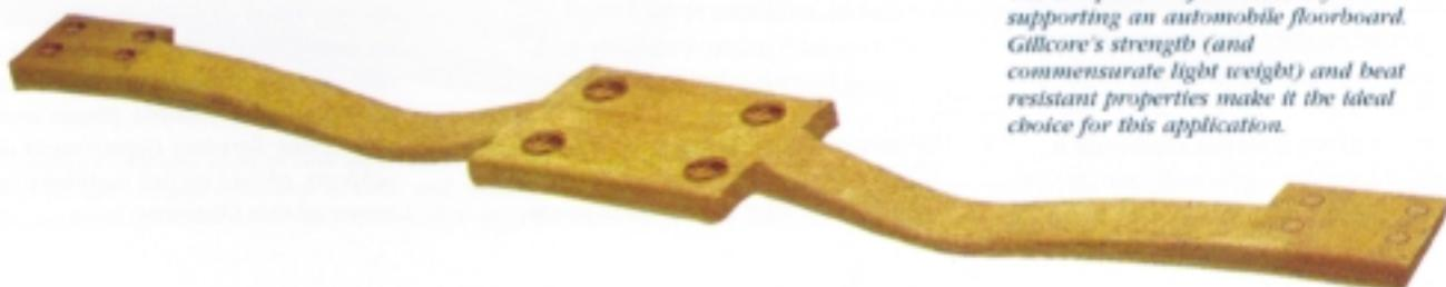
Molded 11 pcf Gillfoam which will ultimately serve as the core material for a structural "beam" that will be one component of an assembly supporting an automobile floorboard. Gillcore's strength (and commensurate light weight) and beat resistant properties make it the ideal choice for this application.
