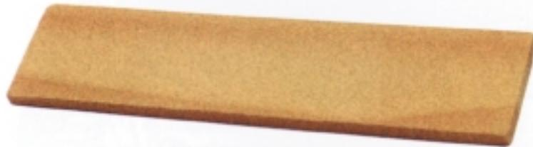
Slice of cured Gillfoam with a density of 1.3 pcf. The ability to manufacture Gillfoam in a wide range of densities make it highly suitable for sandwich panel cores or as a stand alone material.
