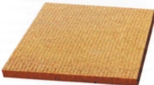
A slice of Nomex honeycomb with Gillfoam-filled cells. The result is a material with greatly improved acoustical and insulating properties, and higher compression and shear strength. The honeycomb slices can be cut to virtually any thickness. Typical applications would include sound deadening bulkheads of marine vessels; temporary or permanent partitions in offices, laboratories and other architectural environments; and, sandwich panel cores in refrigerated railroad cars and trucks.
