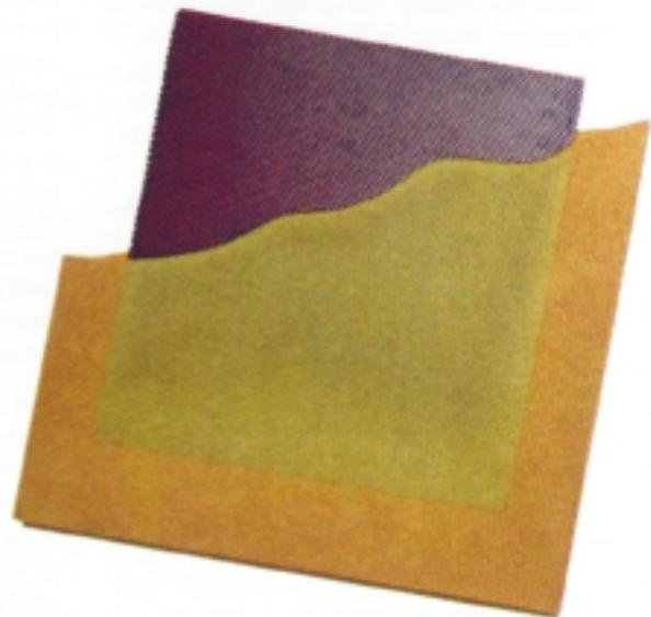
Cutaway view of a phenolic reinforced fiberglass cloth faced, Nomex honeycomb core sandwich panel using 18 pcf Gillfoam as an edge close out. Foam closeouts represent a considerable savings in time and money over routing and putting the edges with a standard two-part epoxy compound.
