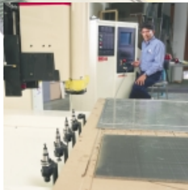
The tool storage bar at the back holds five tools. Programmed in advance, the router head automatically selects the proper tool.
