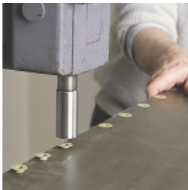
The panel is adjusted on a roller table to ensure proper alignment of inserts. The inserts then are set into the panel.
