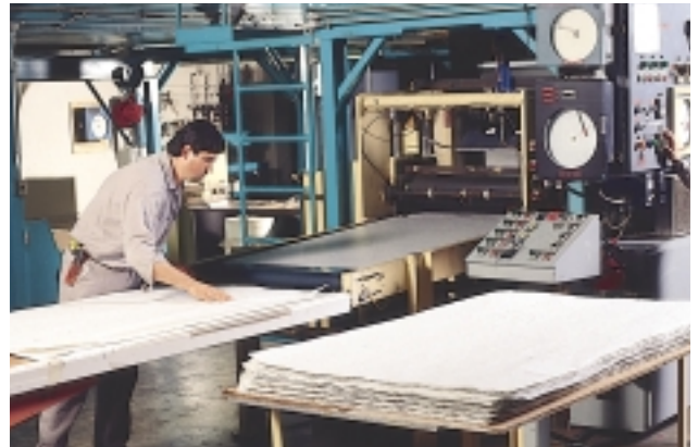
4. The printed paper comes out of the printer conveyor where it is automatically cut off in sheets and stacked, preparatory to inspection and loading into the press.
