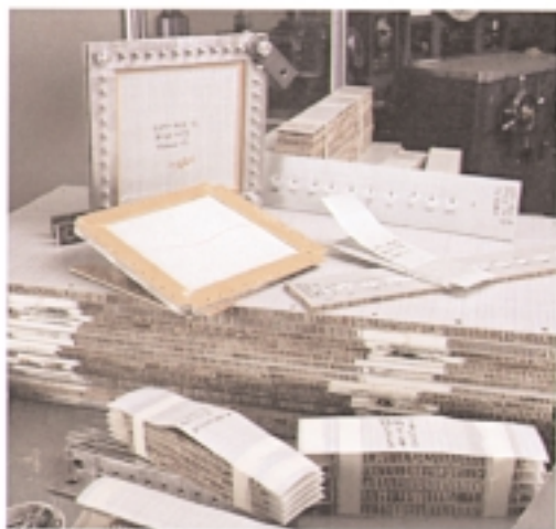
More test samples consisting of some that have already undergone testing and have been bundled and marked for retention; others placed in test fixtures; and, some raw stock still requiring further preparation.
