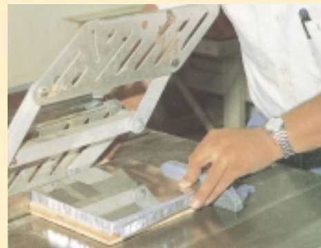
This panel is being cut on a table saw using a carbide tip blade with a backing piece (plywood) under the panel.
