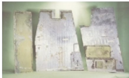
These corroded aluminum flooring panels were removed from the galley of a DC9. This amount of corrosion is typical for aluminum in "wet" areas.
