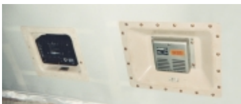
Ceiling-mounted smoke detection unit (right) and a central electronic unit (the black box on the left) shown prior to installation of the wire grid. If smoke is detected, one of the detection units transmits a signal to the central electronic unit which in turn sends the signal on the cockpit, thus alerting crew members.
