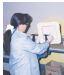
Press operator performs routine wall thickness check with a micrometer.
