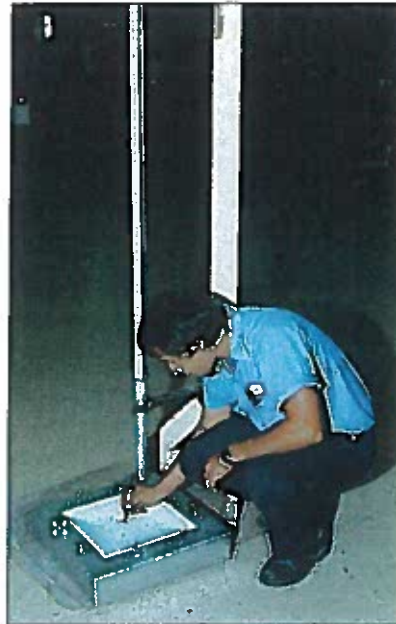
Impact or Puncture Resistance Test indicates the cargo liner's ability to withstand penetration
