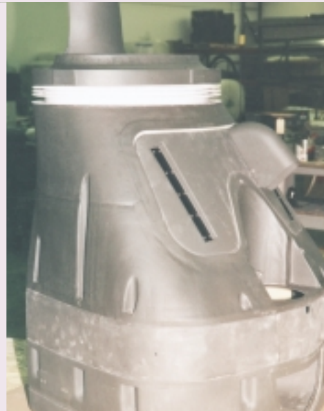
One of two air cleaners for the Blackhawk helicopter; constructed of fiberglass reinforced epoxy and urethane foam.
