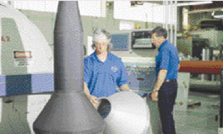
BDA Rx antenna f or a Global Positioning Satellite II, constructed from cynate ester/quartz filament wrapped with dindretic copper.
