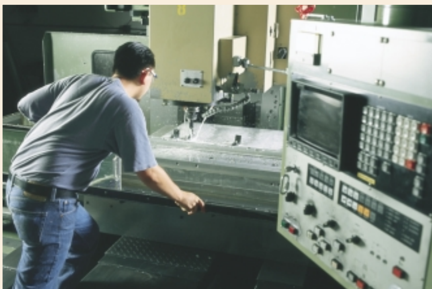
FANUC computer-controlled high speed mill profiling aluminum fittings.
