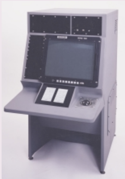
An avionics equipment cabinet-part of the Royal-developed RP900 modular composite cabinetry.
