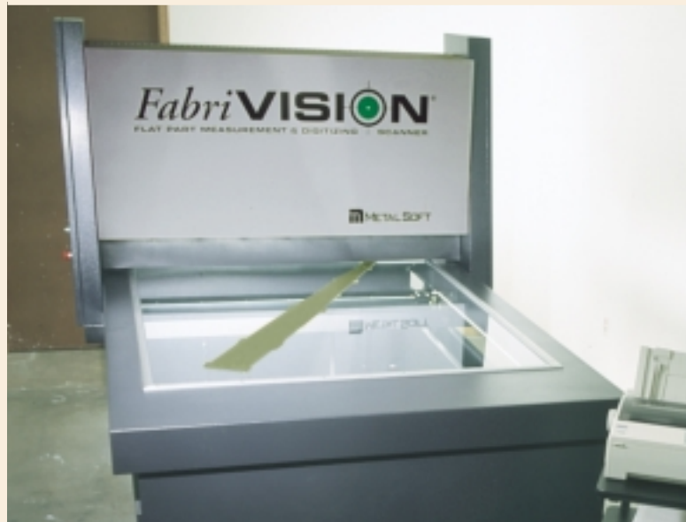
This state-of-the-art dimensional inspection scanner confirms tolerances as tight as \pm .002" .
