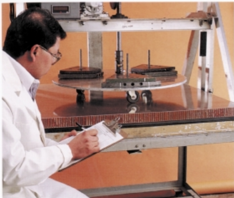
Roller Cart Test measures the fatigue resistance of floor panels including honeycomb core. (The clear skin was used for photographic clarity).
