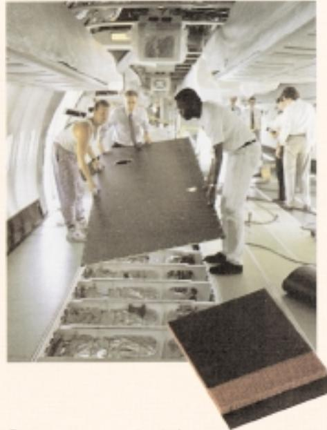
Galleys use Gillfab 4022 panels of low smoke woven fiberglass cloth reinforced phenolic facings with Nomex honeycomb core. Replaced heavier conventional metal and thermoplastic panels. Properties: 1. Specific strength, 3. Low water absorption, 4. Dent resistance, 11. Puncture resistance, 15. Chemical resistance.
