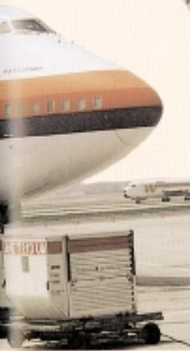
The walls of these LD-3 cargo containers use Gilliner® 1066 fiberglass cloth reinforced polyester laminates. Replaced aluminum. Properties: 1. Specific strength (saves weight), 4. Dent resistance, no flare/shatter, 11. Puncture resistance.
