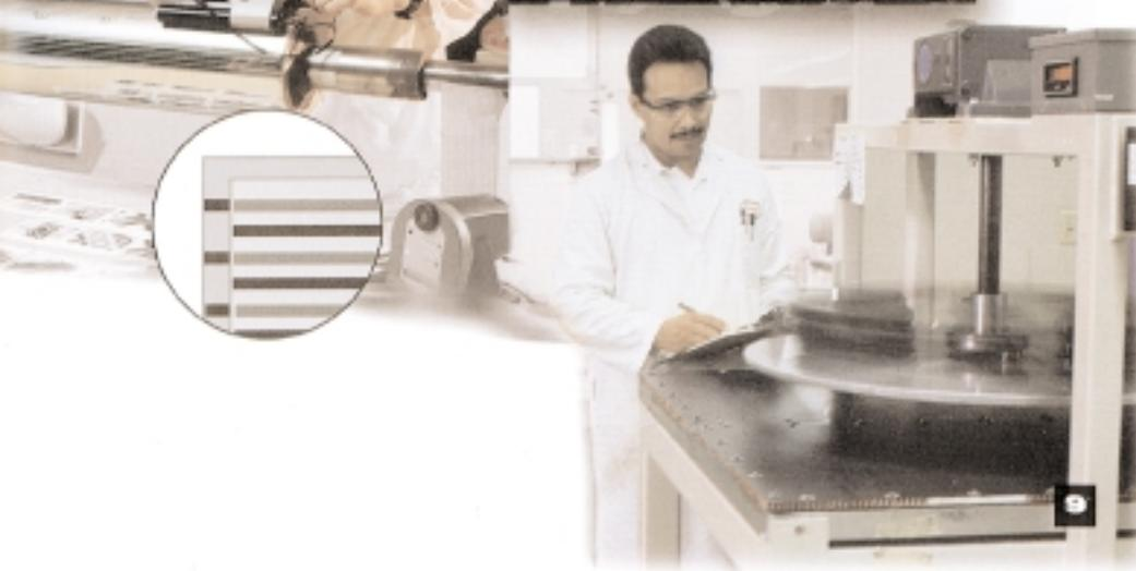
8. This "rolling car" tests fatigue resistance of aircraft flooring panels' core. One specification requires weights of up to 120 pounds on each of the tester's three wheels for 120,000 cycles, and then 158 pounds per wheel for an additional 35,000 cycles. Increased fatigue resistance results in products with lower replacement rates.
