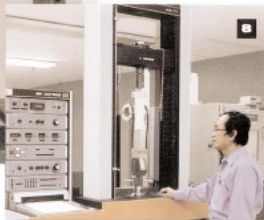
3. The NIST (NBS) smoke chamber measures the smoke emissions of materials exposed to heat and flame. It allows for selection of low smoke density, and therefore safer materials.
