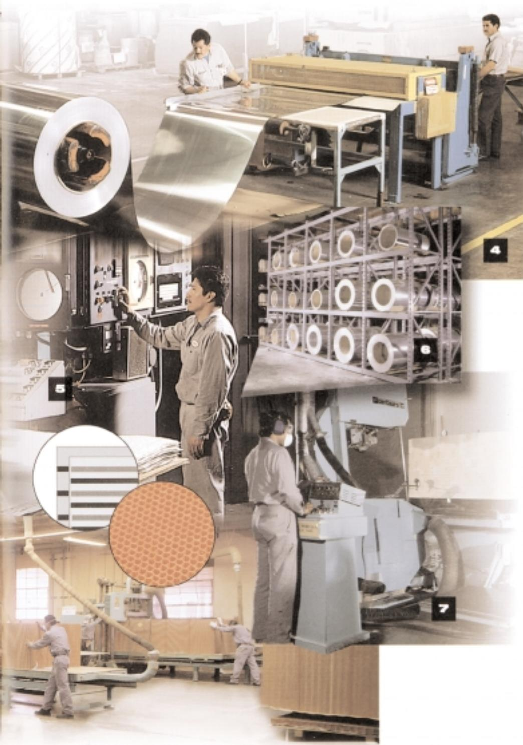
3. Nomex honeycomb loaves are sliced by computer controlled horizontal band saws. They cut loaves up to 60" wide to virtually any thickness with a  $\pm .005"$  tolerance over the entire slice. Cutting our in-house manufactured core and facings helps ensure quality and delivery commitments.
