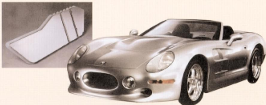
Flooring panels for Carroll Shelby's Series One Cars are made from Gillfab 4030 aluminum honeycomb core and aluminum facings. Replaced aluminum plate.
