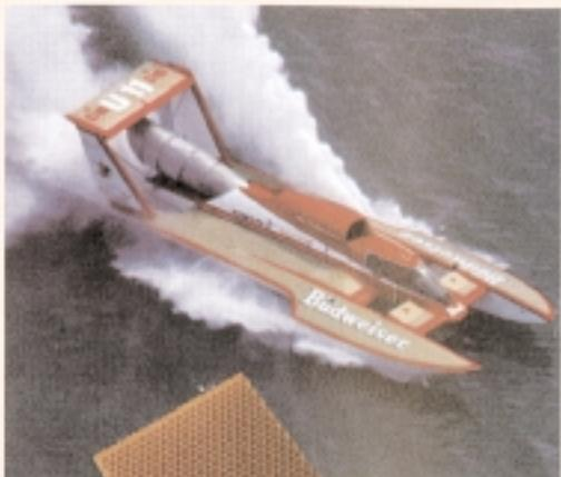
Fiberglass-faced Gilcore® HD (Nomex® honeycomb) is used in the sponsons of this racing boat. Replaced marine plywood / fiberglass facings sandwich panels.
