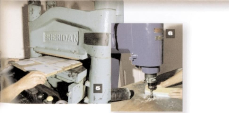
4. This 14' precision shear is used for trimming fiberglass laminates or sandwich panel facings such as composites, aluminum, stainless, or cold-rolled steel.
