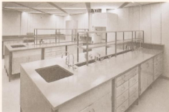
Laboratory counter tops and sinks made from Gillab® 990C polyester reinforced with chopped strand fiberglass mat. Replaced high pressure laminate, ceramic, stainless steel, painted chemical resistant board, or treated plywood because of its chemical resistance. Properties: 3. Low water absorption, 13. Self extinguishing and abrasion resistance, 15. Chemical resistance, 16. Aesthetics.
