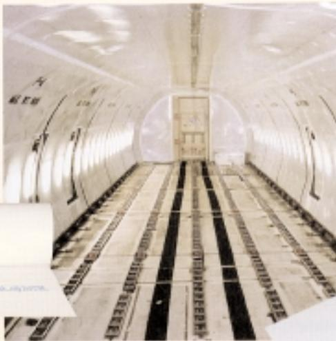
Also, Gillfab 5433C baggage compartment flooring of aluminum facings and epoxy resin impregnated fiberglass cloth core. Replaces solid aluminum sheet. Properties: 1. Specific strength, 4. No flare, 8. Low smoke, 11. Puncture resistance, 13. Self extinguishing. Note: Gillfab 5033 is a similar product, but innovative and lighter because of its resin impregnated Kevlar cloth core.
