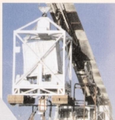
Gillfab 986 is used for spring legs (shown in blue) on shaker machines that shake out large particles from clay in moulding laundry fixtures. These legs were still going strong after 300,000,000 cycles (vs 75,000,000 for steel). Made of epoxy-unidirectional fiberglass rovings. Replaced legs made of steel. Properties: 3. Fatigue proof.
