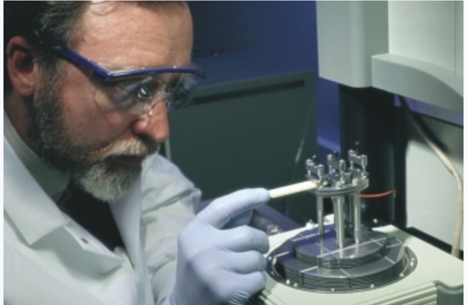
The dynamic mechanical analyzer determines the mechanical properties of material as a function of temperature. Dr. Terry Creasy, Assistant Director of the Composite Center, demonstrates the loading of the sample.
