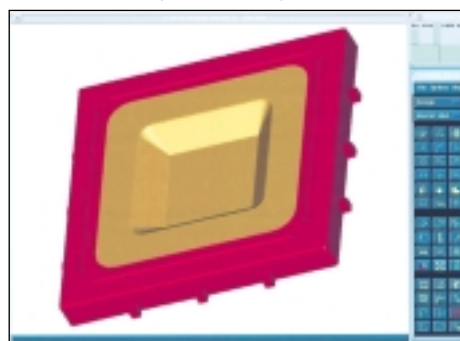
Step 2: Form the tool from the pattern.
