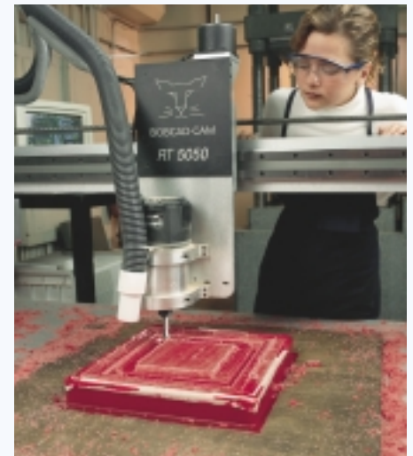
This CNC profiler is used to make tooling and patterns for contoured parts. The operator, Ms. Siari Sosa, is a Ph.D. candidate.
