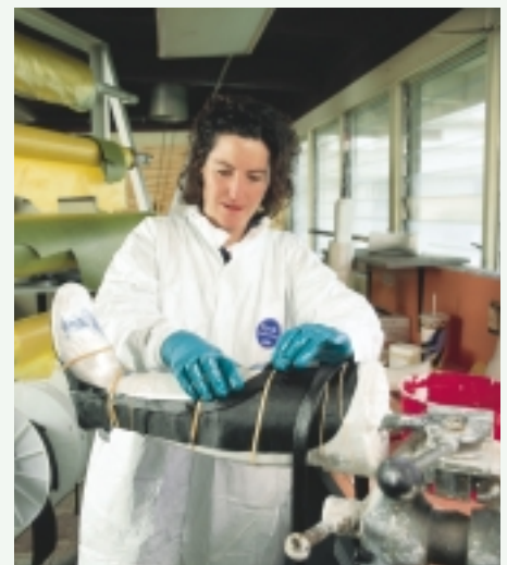
Rancho Los Amigos orthotist Carin Caves laying up a carbon brace on a mold of the ultimate user’s leg.
