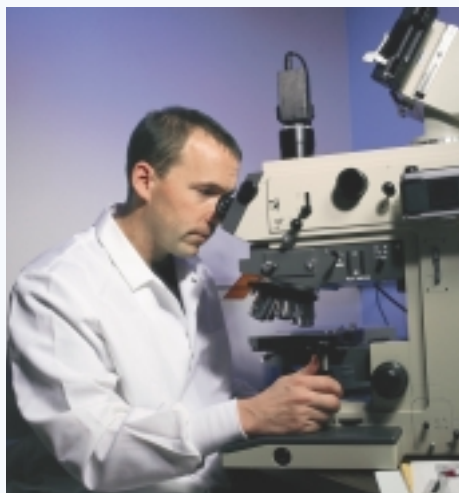
This high-power light microscope allows maximum magnification of polished polymer and composite samples through one of the five turrets. A real-time digital camera captures images for immediate analysis of parameters such as fiber volume fraction.
