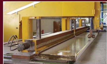
Sawing aluminum honeycomb block before expansion.
