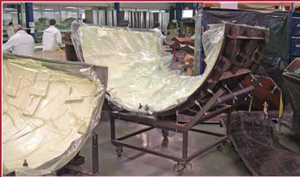
Precision Process Shop (PP2) prepares heat-formed parts for engines' inner-fixed structures.
