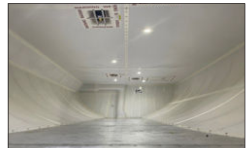
Cargo bay with Gilliner® 1567A sidewalls and ceiling.
