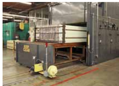
Upgraded heat-set oven to increase capacity.
