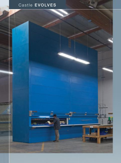
The B787 contract dictates Castle build "buffer stock," so a reorganization of the production floor allowed for the installation of two Kardex vertical carousels. These storage carousels free up valuable floor space and provide a quick and simple solution to managing and storing the buffer stock.
