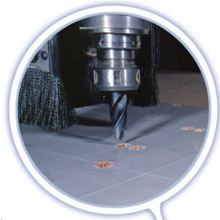
CNC head, drilling and countersinking insert holes.
