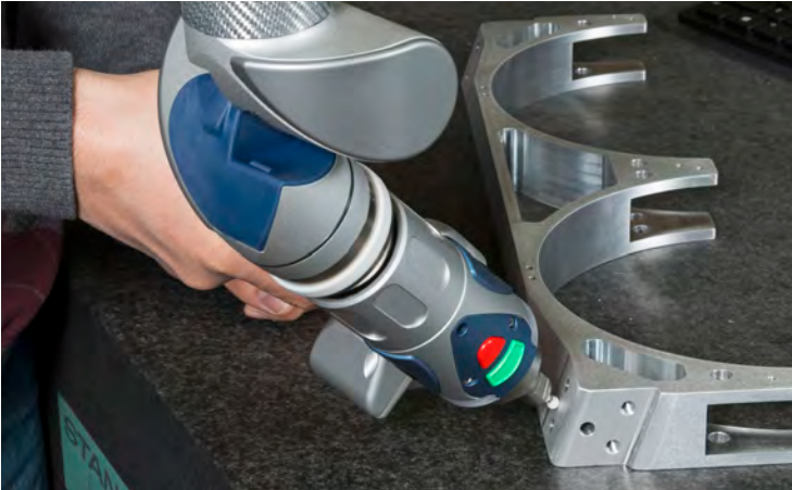
Faro Inspection Arm Measuring an Aluminum Hog-Out
