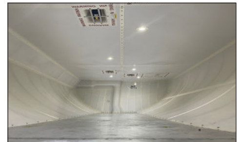
Cargo bay with Gilliner® 1568B sidewalls and ceiling.
