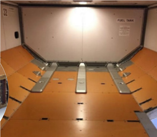
TGC floor and sidewall panels installed on an Airbus A320 aircraft. Photo courtesy of Aeroco Group
