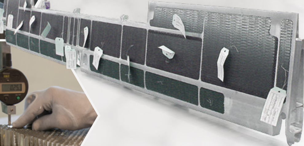
5-Axis machined core inspected in customer frame
