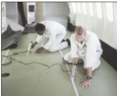
McDonnell Douglas switched from fiberglass-faced flooring panels to carbon and reduced weight in each MD-11 by approx. 350 lbs.
