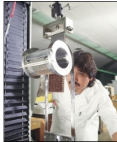
The climbing drum peel test measures force required to separate facing from core; also strength of the adhesive.
