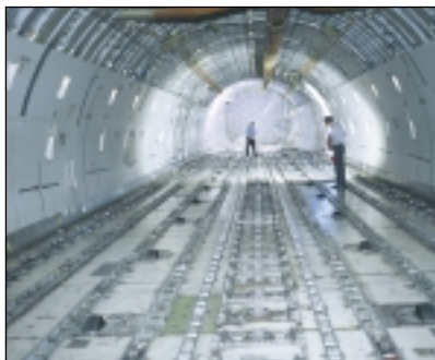
Fiberglass faced/balsa core 5007C sandwich panels for flooring resist high abuse in Federal Express 747 cargo compartments.
