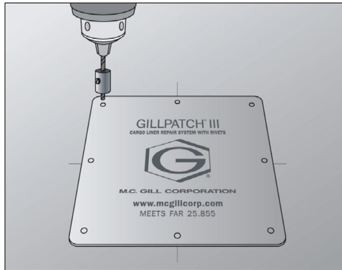
Figure 5 – Drilling Holes in Liner Panel
