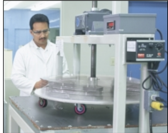
Roller cart test fixture testing a Gillfab 4605 flooring panel, carbon facings with a Nomex Honeycomb core.
