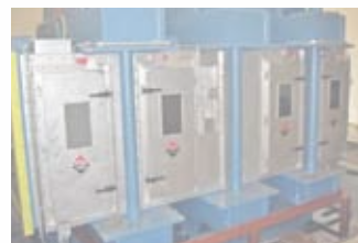
A new press for curing honeycomb blocks.
