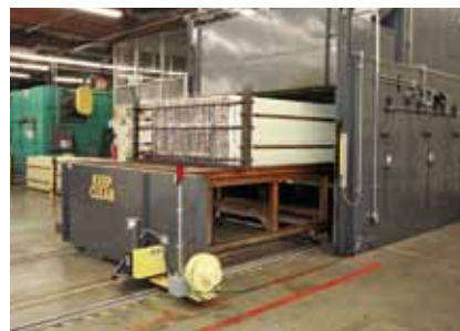
Upgraded heat-set oven to increase capacity.
