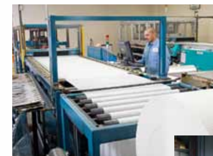
New sheeter/stackers using an advanced Vision system that stacks honeycomb blocks faster and more accurately.
